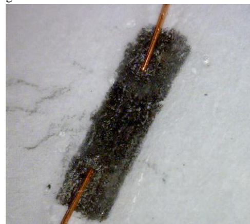
Fig. 2: Digital photograph of piezoresistor graphite on paper.
